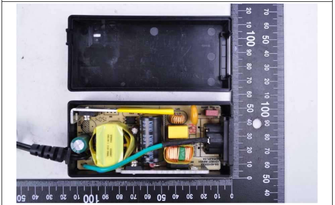
for C14 Inlet type (Earthing wire and output fixed by glue)
